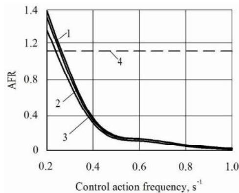
**Figure 6.** Amplitude-frequency characteristic of dynamic system's response to control action at different values of the design parameter  $l_2$ : 1) 3.15 m; 2) 2.15 m; 3) 4.15 m; 4) desirable (ideal) amplitude-frequency characteristic.
