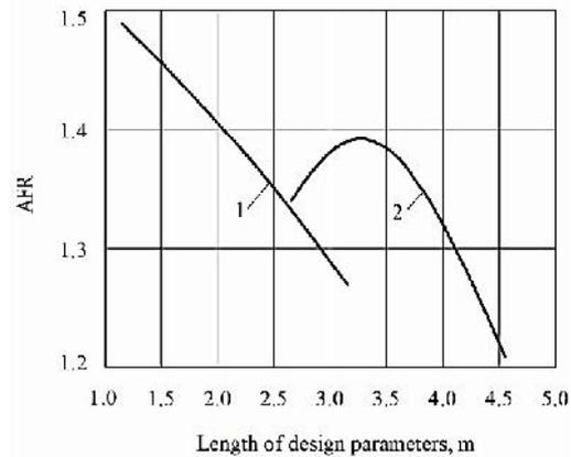
**Figure 7.** Amplitude-frequency characteristics of dynamic system's response to control action at a frequency of  $0.2 \text{ s}^{-1}$  at different values of the design parameters  $\alpha_2$  (1) and  $l_2$  (2).
