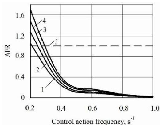
**Figure 3.** Amplitude-frequency characteristic of dynamic system's response to control action at different values of coefficient of rolling resistance: 1) 0.10; 2) 0.12; 3) 0.14; 4) 0.16; 5) desirable (ideal) amplitude-frequency characteristic.
