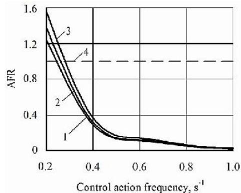
**Figure 5.** Amplitude-frequency characteristic of dynamic system's response to control action at different values of the design parameter  $\alpha_2$ : 1) 1.15 m; 2) 2.15 m; 3) 3.15 m; 4) desirable (ideal) amplitude-frequency characteristic.
