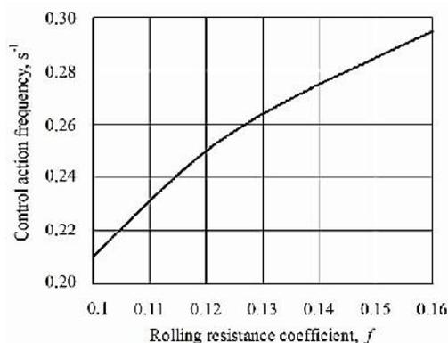
**Figure 4.** Relation between the desirable frequency of angular displacement of steering wheels of combine tractor in combined fertilising and sowing tractor-implement unit and the conditions of its motion (coefficient of rolling resistance  $f$ ).
