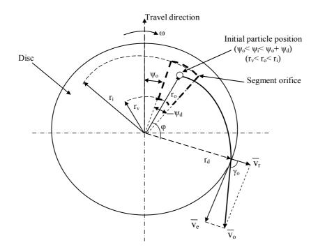
Fig. 1. Parameters of particle position.
