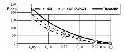
**Fig. 3.** The dependence of the disc turning angle  $\varphi$  on the radius  $r_0$  when the particle gets on the disc:  $-\mathbf{x} - \varphi = -91 \ln(r_0) - 117,16$ ;  $R^2 = 0,99$ ;  $-\Delta - \varphi = -105,6 \ln(r_0) - 133,88$ ;  $R^2 = 0,99$ ;  $-\Box - \varphi = -125,57 \ln(r_0) - 153,48$ ;  $R^2 = 0,99$
