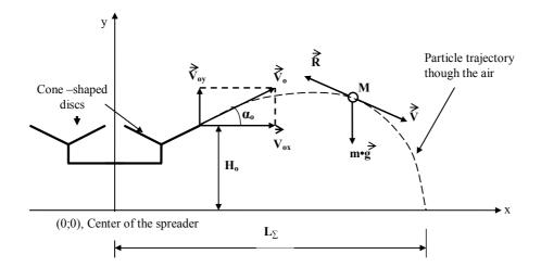
Fig. 2. Particle trajectory though the air
