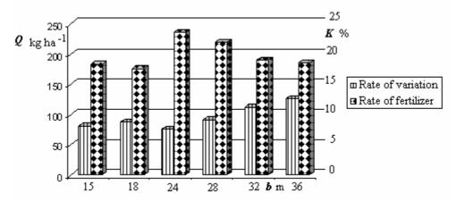
**Fig. 6.** The dependence of the rate of variation K (%) and the rate of fertilizer Q (kg ha<sup>-1</sup>) on the width of lot b (m).
