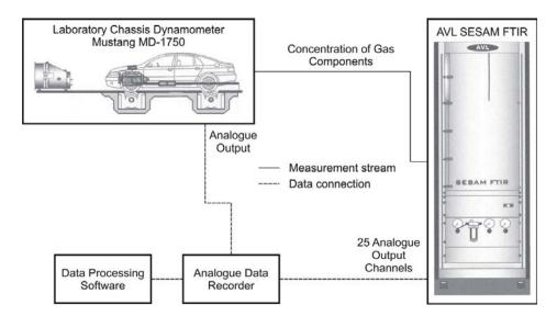
Fig. 2. Block diagram of the emission test routines.
