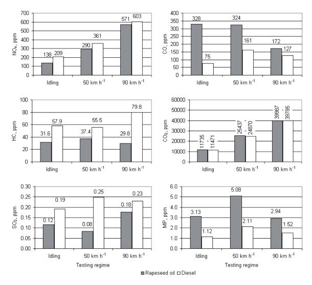
The results of exhaust emission analysis for automobile MAN 19,464, rebuilt to run on rapeseed oil with a two-tank system, are shown in Fig. 4.
