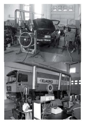
Fig. 1. Vehicles used in the experiments (VW Golf 1.9TDI and MAN 19,464).
