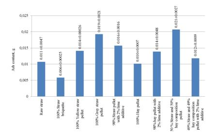
Figure 2. Ash content in tested samples.
