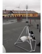
**Figure 3.** Vaisala weather station MAWS201 and 300 W wind generator.
