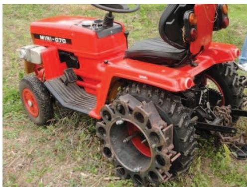
**Figure 3.** The tractor type Mini 070 equipped with standard tires and special wheels.
