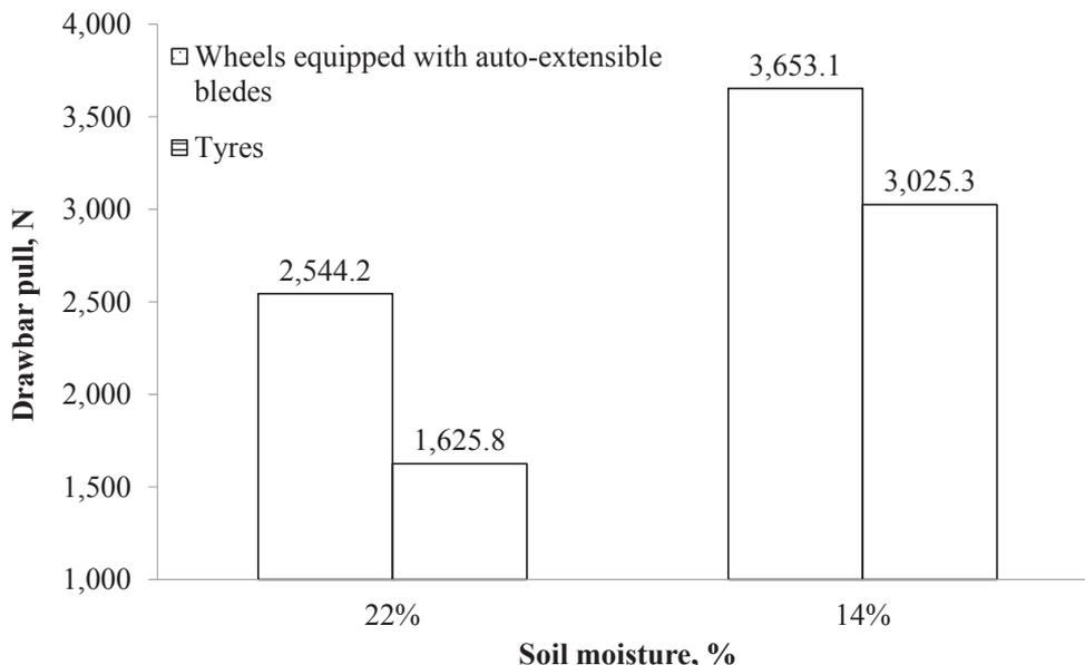
**Figure 7.** The final comparison of special wheels and tyres installed in tractor.
