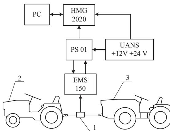
**Figure 2.** System for measurement of tractor drawbar pulls: 1 – force sensor EMS 150, 2 – tractor type Mini 070 equipped with different wheel types, 3 – loading tractor type T4K10, HMG 2020 – digital portable recording device, UANS – universal battery source, PC – personal computer, PS 01 – junction box.
