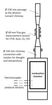
**Figure 1.** Illustration of the test bench with a flue gas measurement section (hot) for the emission measurement.
