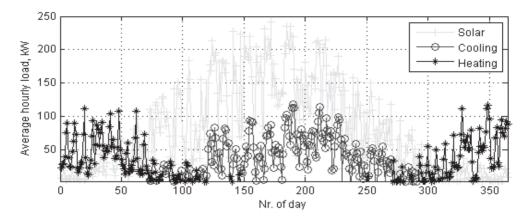
**Figure 3.** Heating, cooling, hot water and electrical loads and solar irradiation of the longer side of a south oriented office building.
