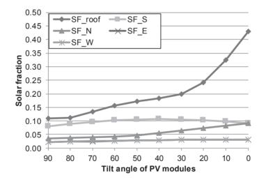
Figure 7. Solar fraction of four facades and the roof to the total energy consumption.
