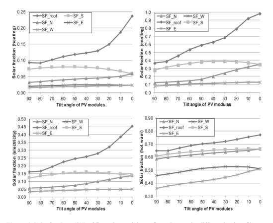
**Figure 6.** Solar fractions (SH) of five solar module configurations under different load profiles – heating, cooling, electricity, and hot water. Every line depicts results for north (N), east (E), south (S), west (W) facades or the roof.
