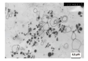
**Figure 1.** Electron microscopy image of ultra-thin slice of beta-carotene loaded liposomes in the dairy product matrix on the first day of storage.
