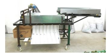
Figure 1. Model of roller conveyor.
