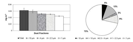
**Figure 4.** Concentrations and percentage of size distribution of dust fractions inside the office C after the wiping of the floor  $C_2$ .
