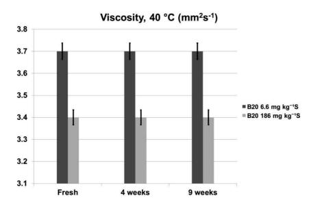
Figure 1. The results of viscosity measurements.
