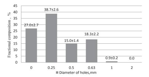
Figure 5. Fraction composition of fibre nettle mill.
