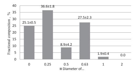
Figure 4. Fraction composition of fibre hemp Epsilon 68 mill.
