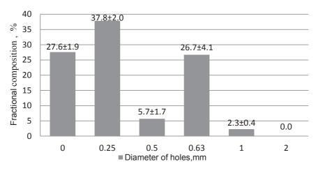
Figure 2. Fraction composition of fibre hemp Beniko mill.
