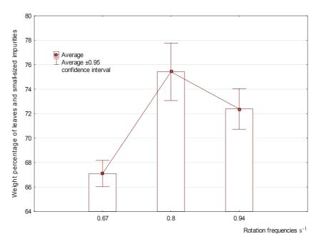
**Figure 10.** Weight percentage of leaves and small-sized impurities in the waste with the rollers of 89 mm in diameter, gap of 24 mm and three rotation frequencies.
