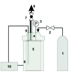
**Figure 1.** Schematic of the explosive decompression pretreatment system: 1 – nitrogen tank; 2 – pressure control valve; 3 – manometer; 4 – modified reactor vessel cap; 5 – reactor vessel; 6 – ceramic contact heater; 7 – pressure release valve; 8 – into ventilation system; 9 – thermocouple; 10 – controller unit.
