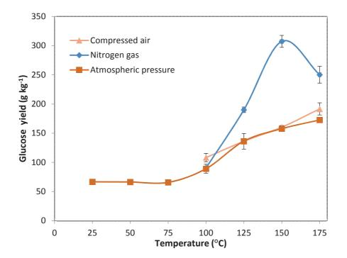
**Figure 2.** Comparison of glucose yields gained at pressure of 30 bars with different pretreatment methods when the pretreatment temperature was gradually increased.
