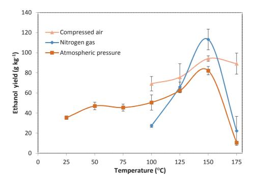
Figure 4. Comparison of ethanol yields gained with different pretreatment methods at 30 bars and at near atmospheric pressure when the pretreatment temperature was gradually increased.
