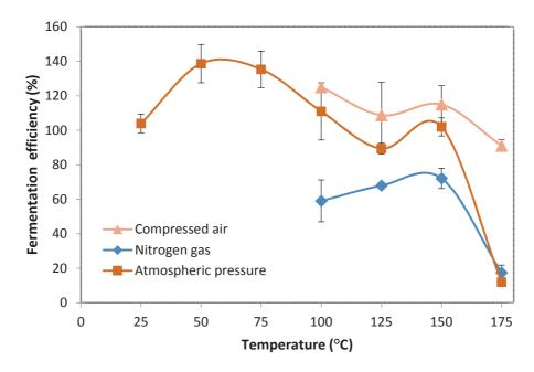
**Figure 5.** Comparison of fermentation efficiencies gained with different pretreatment methods at 30 bars or at atmospheric pressure when the pretreatment temperature was gradually increased.
