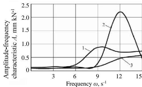
**Figure 12.** Amplitude frequency response characteristic of vertical oscillations of tractor's rear axle, when it responds to variation of rear-mounted plough's tractive resistance at different coefficients  $C_{tP}$ : 1 –  $250 \text{ kN m}^{-1}$ ; 2 –  $350 \text{ kN m}^{-1}$ ; 3 –  $450 \text{ kN m}^{-1}$ .
