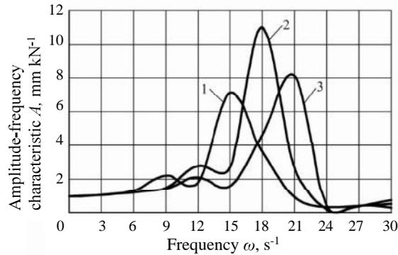
**Figure 6.** Amplitude frequency response characteristic of vertical oscillations of front axle of tractor, when it responds to variation of soil surface profile at different stiffness coefficients of tyres on its wheels  $C_T$ : 1 – 250 kN m<sup>-1</sup>; 2 – 350 kN m<sup>-1</sup>; 3 – 450 kN m<sup>-1</sup>.
