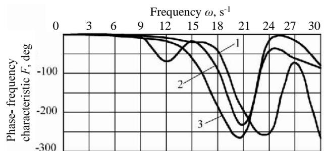
**Figure 7.** Phase frequency response characteristics of vertical oscillations of front axle of tractor, when it responds to variation of soil surface profile at different stiffness coefficients of tyres on its wheels  $C_T$ : 1 – 250 kN m<sup>-1</sup>; 2 – 350 kN m<sup>-1</sup>; 3 – 450 kN m<sup>-1</sup>.
