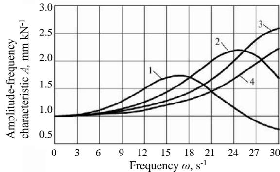
**Figure 9.** Amplitude frequency response characteristics of vertical oscillations of chopper's frame, when it responds to variation of soil surface profile at different tyre stiffness coefficients  $C_{tG}$ : 1 –  $50 \text{ kN m}^{-1}$ ; 2 –  $100 \text{ kN m}^{-1}$ ; 3 –  $150 \text{ kN m}^{-1}$ ; 4 –  $200 \text{ kN m}^{-1}$ .
