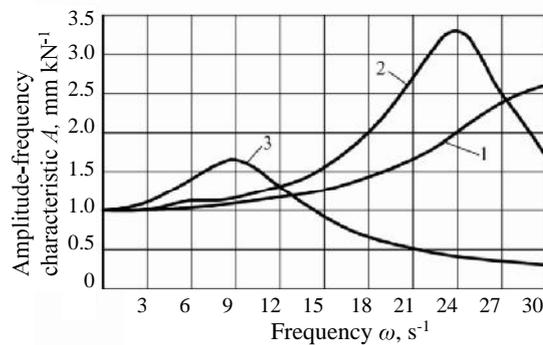
**Figure 10.** Amplitude frequency response characteristic of vertical oscillations of chopper's frame, when it responds to soil surface profile variation at different masses  $M_G$  and tyre stiffness coefficients  $C_{tG}$ : 1 –  $M_G = 300 \text{ kg}$ ;  $C_{tG} = 150 \text{ kN m}^{-1}$ ; 2 –  $M_G = 500 \text{ kg}$ ;  $C_{tG} = 150 \text{ kN m}^{-1}$ ; 3 –  $M_G = 300 \text{ kg}$ ;  $C_{tG} = 25 \text{ kN m}^{-1}$ .
