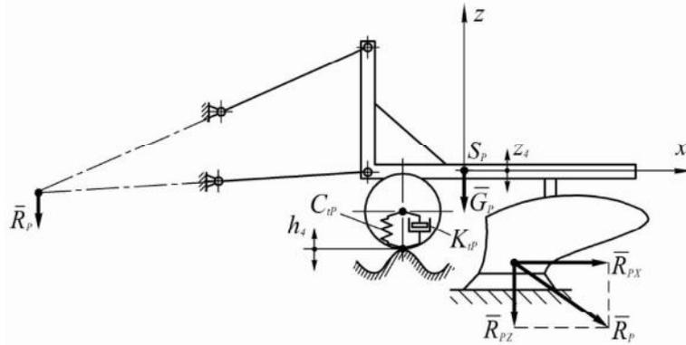
**Figure 4.** Equivalent schematic model of vertical oscillations of plough that is rear-mounted on tractor.
