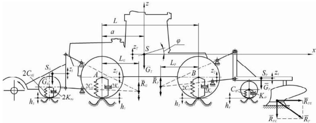
**Figure 1.** Equivalent schematic model of the combined chopping and ploughing tractor-implement unit in the longitudinal and vertical plane.
