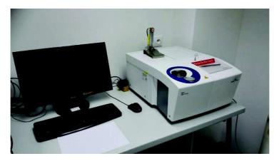
Figure 1. Mettler Toledo DSC unit.
