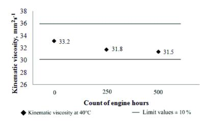
Figure 2. Kinematic viscosity at 40 °C during operating test.
