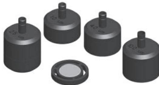
**Figure 2.** Impactors for PM<sub>10</sub>, PM<sub>4</sub>, PM<sub>2.5</sub>, PM<sub>1</sub> measurement.
