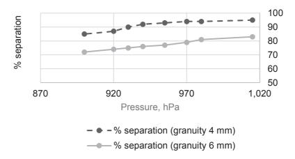
Figure 2. The dependence of separation efficiency on the operating pressure 6 mm mesh.
