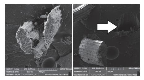
Figure 5. Fracture areas of sisal composites systems (SEM).
