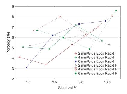
Figure 2. Porosity of Epoxy/Sisal composites.
