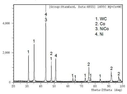
Figure 9. The XRD analysis (Ni-Co-WC) composite Sintered in tube furnace at 1,400 °C.
