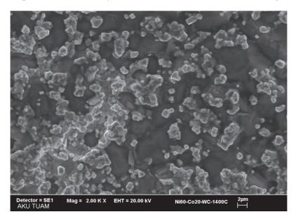
Figure 4. SEM view of (Ni-Co-WC) composite 1,400 °C.
