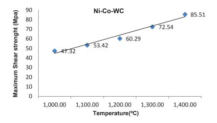
Figure 3. Shear strength results from specimens sintered at different temperatures.
