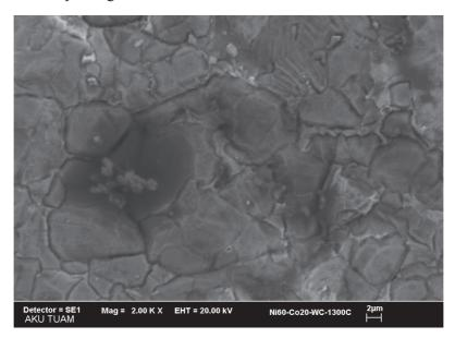
Figure 5. SEM view of (Ni-Co-WC) composite 1,300 °C.
