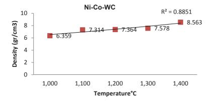
Figure 1. The density change with respect to sintering temperature.
