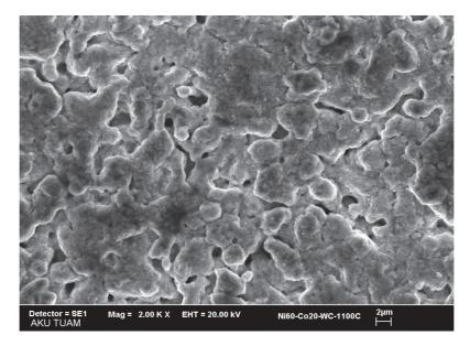
Ni-Co, WC composites are sintered at 1,000  $^{\circ}\text{C}$  , 1,100  $^{\circ}\text{C}$  . The SEM picture Fig. 7 shown some porous unclear phases.
