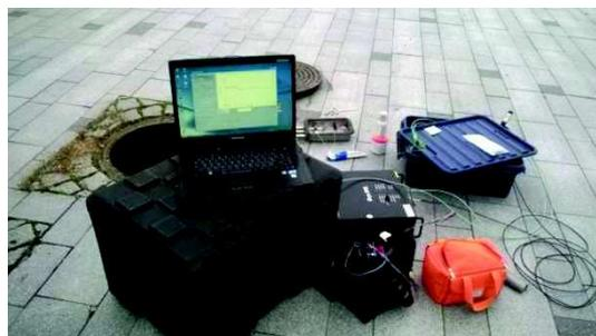
**Figure 1.** DTS-device was in commission at the low energy network site in Suvilahti.
