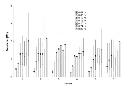
**Figure 4.** Cone index of all variants at Lázně Bělohrad in May, 2015 (mean, minimum–maximum range).
