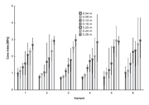
Figure 5. Cone index of all variants at Lázně Bělohrad in April, 2016 (mean, minimum-maximum range).
