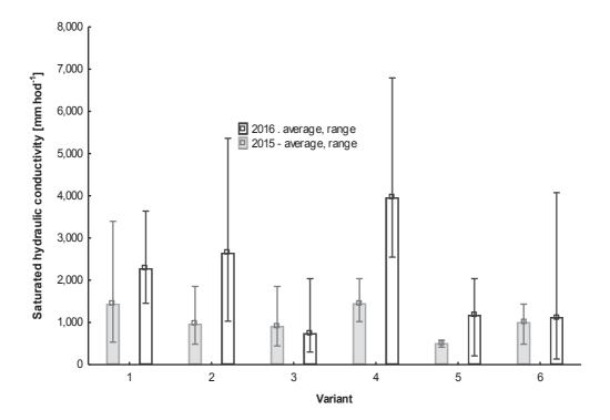
**Figure 2.** Saturated hydraulic conductivity of all the variants at Lázně Bělohrad in May, 2015 and April, 2016 (mean, minimum–maximum range).
