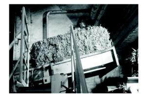
Figure 1. Package of maize cortical inserted into the dosing device of incinerator.
