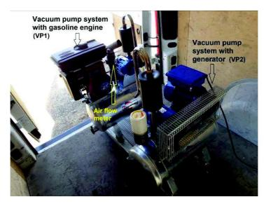
Figure 1. VP1 and VP2 driven by gasoline engine and generator, respectively.
