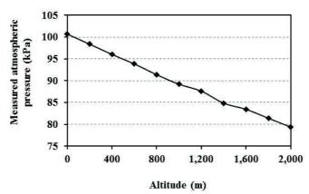
Figure 4. Measured atmospheric pressure as affected by the altitude.
