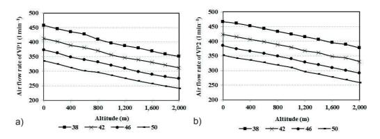
**Figure 7.** The effect of altitude on air flow rate of vacuum pumps at pressure range of 38–50 kPa for VP1 and VP2.
