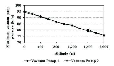
Figure 5. Maximum pressure and altitude relationships of VP1 and VP2.
