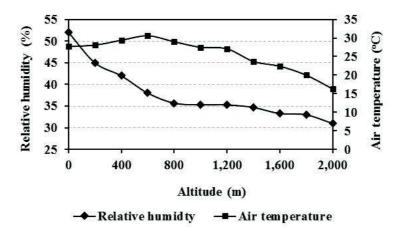
Figure 3. Measured relative humidity and air temperature as a result of altitude change.
