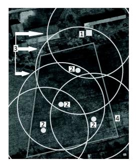
**Figure 1.** Design for wireless network distribution through stationary repeaters (1 – gateway; 2 – stationary repeater; 3 – wireless range, 4 – fence).
