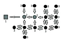
**Figure 4.** The transfer principle for a MESH wireless network (1 – gateway; 2 – stationary repeater; 3 – transmitter).
