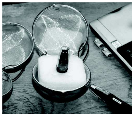
Figure 2. Inserting a data-logger into a protective sieve.
