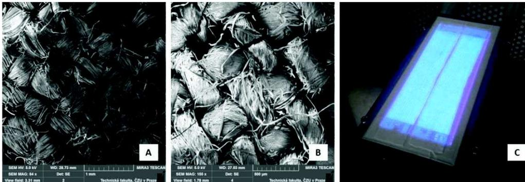
**Figure 1.** Reinforcing phases. A: SEM images of cotton MAG 84 x, B: SEM images of flax MAG 155 x, C: surface treatment of flax using plasma discharge at 350 W.
