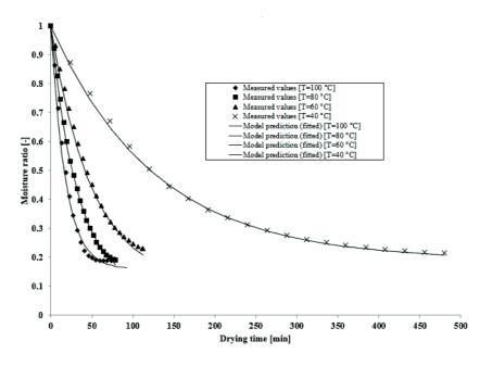
Figure 2. Comparison of measured values of moisture ratio and fitted models in the air temperature range of 40-100 °C.
