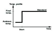
Figure 1. Drying profile: Standard for moisture balance Radwag
