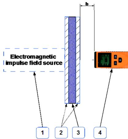
**Figure 3.** Schematics of experimental rig used for local EMF strength measurements: 1 – Source of electromagnetic impulse fields; 2 – Layer made of crumb rubber; 3 – Layer made of crumb rubber – iron powder mixture (CRIP); 4 – Electromagnetic radiation tester-teslameter GM3120.
