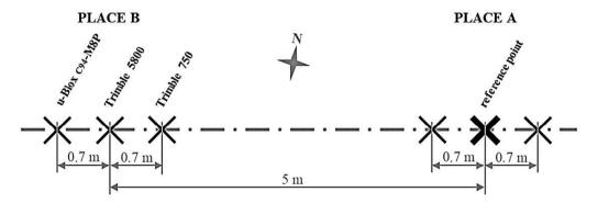
Figure 1. Placement of receiver antennas.
