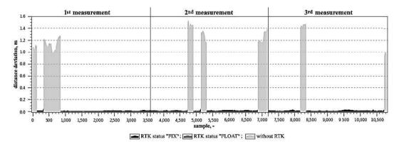
Figure 5. Accuracy deviation and system status of Trimble 750.
