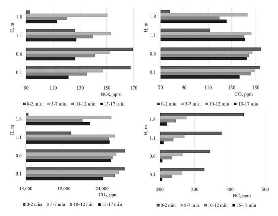
Figure 2. Variation of main regulated emissions (NOx, CO, CO<sub>2</sub> and HC) for diesel engine (Volvo V70 2.5TDI).
