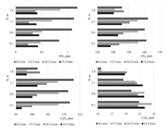
**Figure 5.** Variation of main unregulated emissions (NH<sub>3</sub>, CH<sub>4</sub>, C<sub>2</sub>H<sub>2</sub> and C<sub>2</sub>H<sub>6</sub>) for gasoline engine (Audi A6 2.6).
