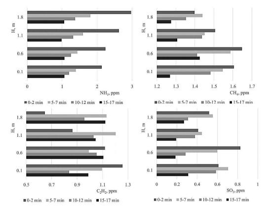
**Figure 4.** Variation of main unregulated emissions (NH<sub>3</sub>, CH<sub>4</sub>, C<sub>2</sub>H<sub>2</sub> and SO<sub>2</sub>) for diesel engine (Volvo V70 2.5TDI).
