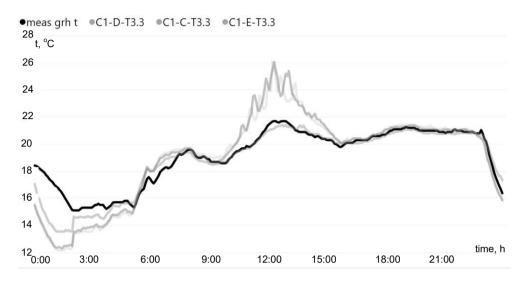
**Figure 6.** uMOL system and greenhouse temperature data comparison using only levels C,D,E (plant area).
