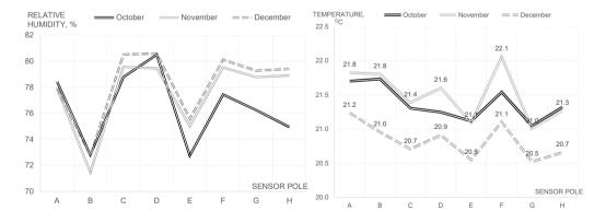
Figure 9. uMOL system monthly average relative humidity (left) and temperature (right) readings per sensor poles A-H.
