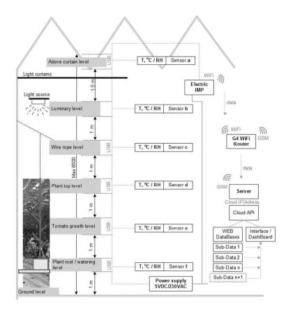
Figure 2. uMOL data system and temperature and humidity sensor pole schematic.
