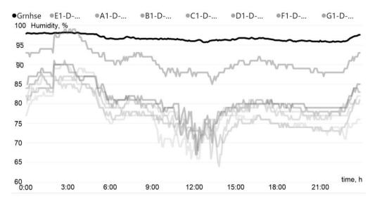
**Figure 8.** uMOL system D level relative humidity readings per poles A-H comparing to humidity deficit values (bold).
