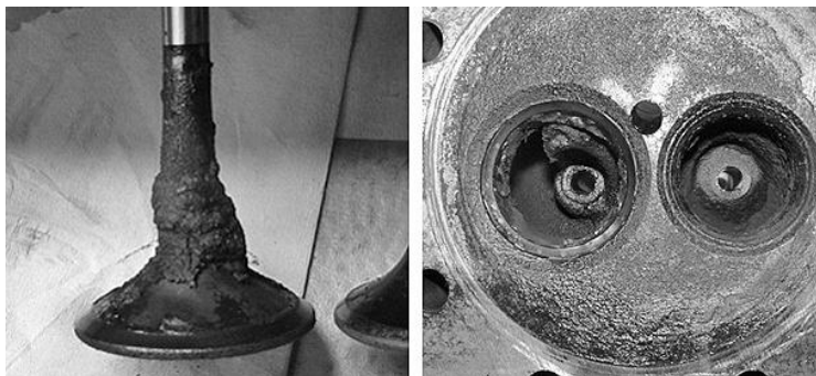
Figure 2. Carbon deposits caused by crude mustard seed oil and rapeseed oil fuels in four cylinder direct injection tractor engine.
