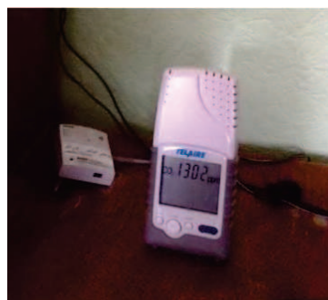
Figure 4. CO 2 sensor Telaire 7001 and data logger Hobo placed in a second floor apartment, 11 Zirnu Street.
