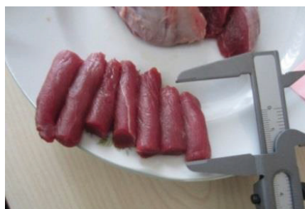
Figure 3. Samples of meat taken by hollow drill.
