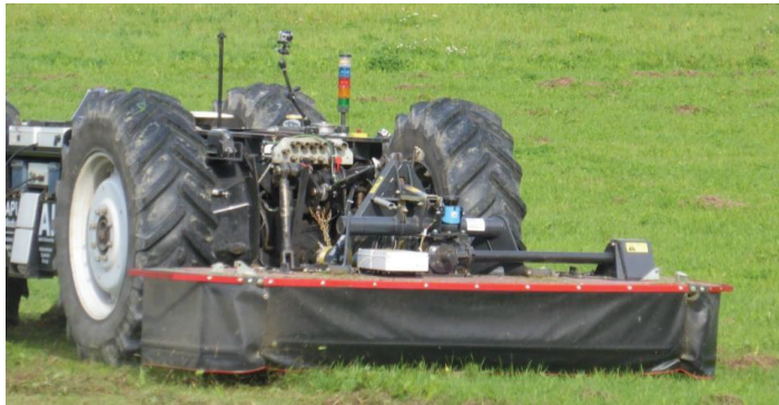
Figure 1. Installation of the laser scanner on the mower. The laser scanner is the blue component in the center.
