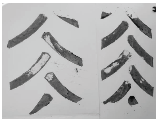
Figure 3. Tyre footprints – left MITAS AC 85, right – MITAS VF (load 4.29 kN).
