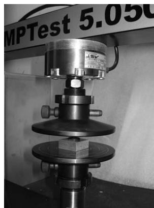
Figure 1. Measurement Compression set.
