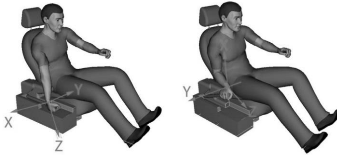
Figure 2. Position of the driver when gripping the handle of the mechanical handbrake with a classic design
