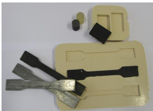
Figure 2. Models for forming, forms, test samples (for testing hardness, tensile strength, abrasive wear).
