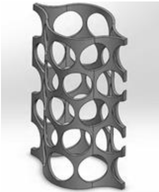
Figure 6. The model of cellular structure basic element.
