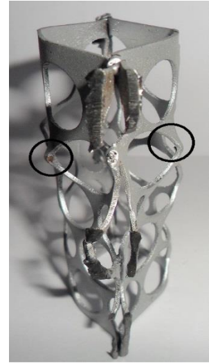
Figure 8. View of deformed basic element of cellular structure and the load bearing capacity local failure places.
