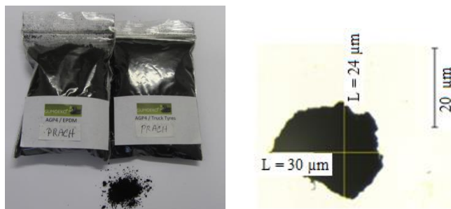
Figure 1. Product from the production line: EPDM rubber powder.
