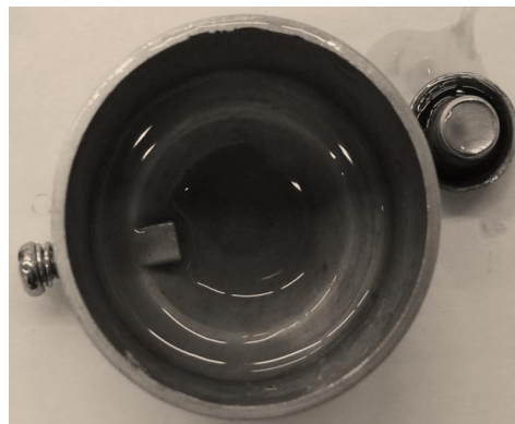
Figure 11. Accumulated oil in carburettor float chamber.
