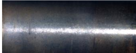
Gen. 2 piston pin, working surface below the bearing.
