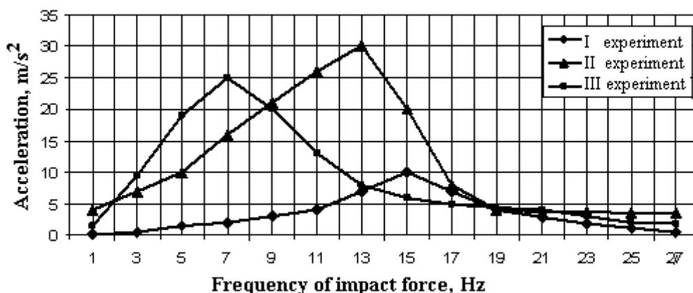
**Fig. 3.** Characteristics of amplitude frequency, while pressing chopped grass forage by directed action vibrator: experiment I – mass of chopped maize; experiment II – mix of maize–goat’s rue; experiment III – chopped goat’s rue.
