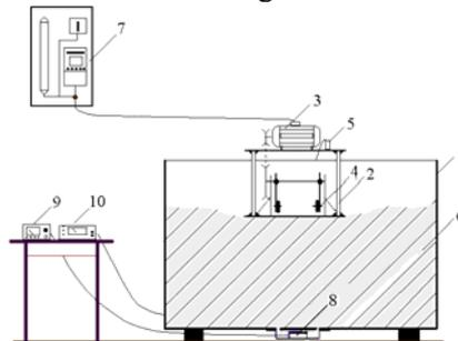
**Fig. 1.** Scheme of grass thickening in container storage using vibratory device: 1 – container storage; 2 – centrifugal-undirected action vibrator; 3 – electrical engine; 4 – changeable weights; 5 – vibration sensor; 6 – mass of thickened grass; 7 – electric current frequency converter; 8 – tensometer sensor; 9 – pressure measurement device; 10 – vibration measurement device.
