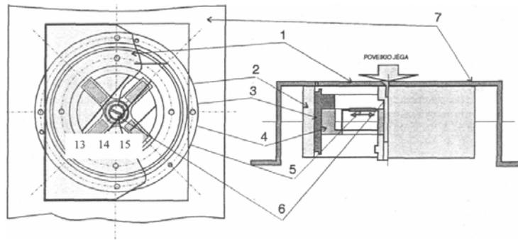
**Fig. 2.** Scheme of tensometer sensor: 1 – sensitive plate; 2 – tensometer body; 3 – tensometer liner; 4 – tensometer membrane; 5 – tenso-converter; 6 – fastening screw of sensitive plate; 7 – tenso-block body.
