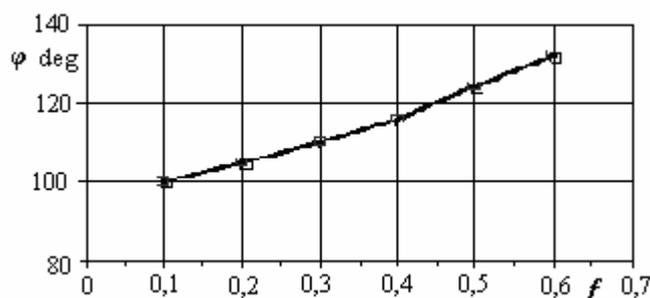
**Fig. 4.** The dependence of the disc turning angle  $\varphi$  on the particle slide friction rate  $f$ :  $\varphi = 62,57 f + 92,60$ ,  $R^2 = 0,98$
