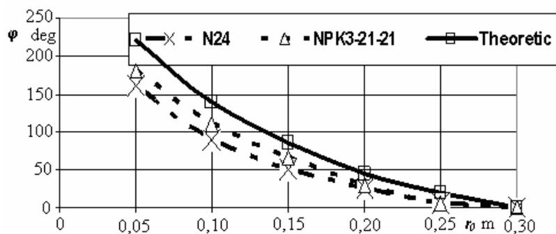
**Fig. 3.** The dependence of the disc turning angle  $\varphi$  on the radius  $r_0$  when the particle gets on the disc: —x—  $\varphi = -91 \ln(r_0) - 117,16$ ;  $R^2 = 0,99$ ; -Δ-  $\varphi = -105,6 \ln(r_0) - 133,88$ ;  $R^2 = 0,99$ ; —□—  $\varphi = -125,57 \ln(r_0) - 153,48$ ;  $R^2 = 0,99$
