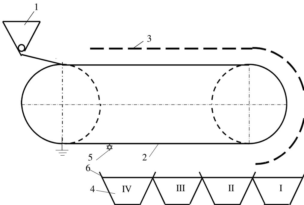
**Fig. 1.** Scheme of the conveyor type electric separator: 1–batcher; 2–conveyor belt (grounded electrode); 3–corona discharge field electrode; 4–reception sizer; 5–brush; 6–partitions between fractions
