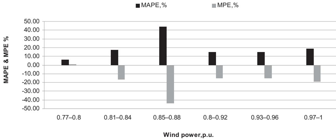
**Fig. 5.** MAPE and MPE of proportional power in Pakri wind park (6/10/2008-12/10/2008 and 3/11/2008-9/11/2008) in interval 0.77-1 by step 0.04.
