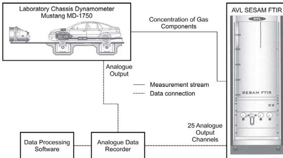
**Fig. 2.** Block diagram of the emission test routines.
