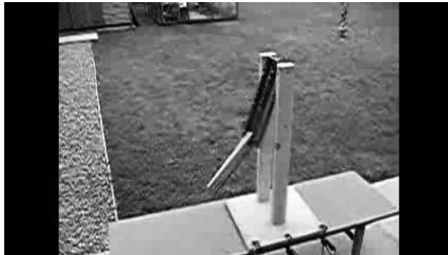
Figure 10. A frame from video clip, showing chaotic oscillation of the physical model of a double pendulum.
