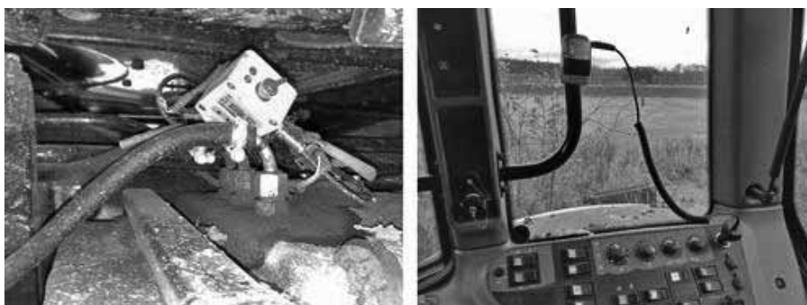
Figure 1. Simple and cost-effective system for determination of the fuel consumption of farm machinery in \text{l ha}^{-1} . System is installed in a Valtra N141 tractor.
