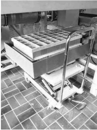
**Figure 5.** Set-up for measuring mass flow distribution at discharge by pilot dryer.
