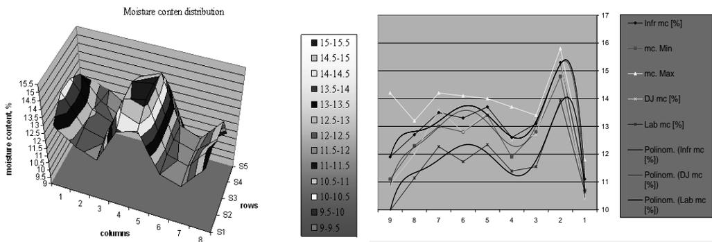
**Figure 7.** Distribution of grain moisture content in the pilot and in the industrial dryer.
