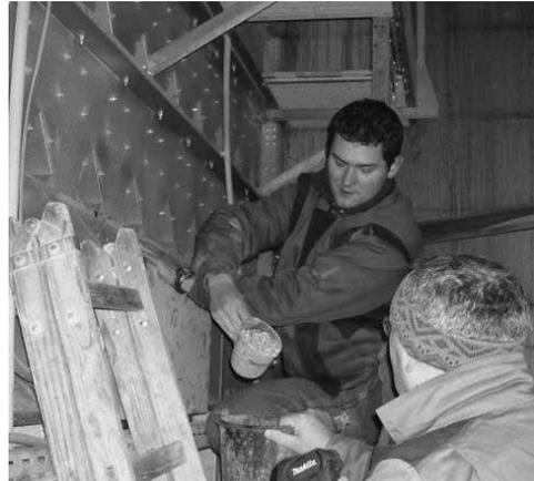
**Figure 6.** Sampling from industrial dryer.
