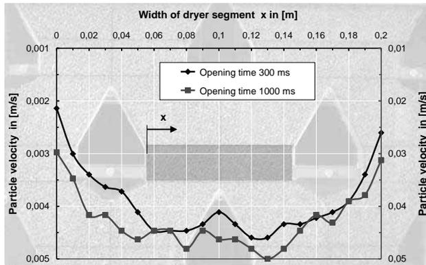
**Figure 2.** Vertical particle velocities measured at the front wall between two air ducts at 300ms and 1,000ms opening time.
