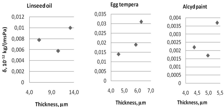
**Figure 3.** Water vapour permeation coefficient depending on the thickness of layers.
