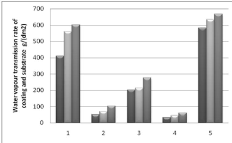
**Figure 1.** Water vapour transmission rate of coating and substrate  $V_{cs}$ , : 1 – casein paint, 2 – linseed oil paint, 3 – egg tempera, 4 – alcyd paint, 5 – carton.
