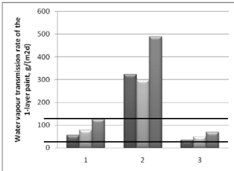
**Figure 2.** Water vapour transmission rate of paints  $V$ : 1 – linseed oil paint, 2 – egg tempera, 3 – alcyd paint.
